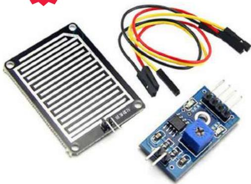
**RAINDROPS SENSOR DE HUMEDAD, SENSIBLE A LA LLUVIA 3.3-5V**
